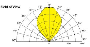
To meet the requirements of EN54:10 clause 5.4, where the ratio of the response points. Dmax: Dmin should not exceed 1.41, the horizontal and vertical viewing angles max should not exceed ±30°.
